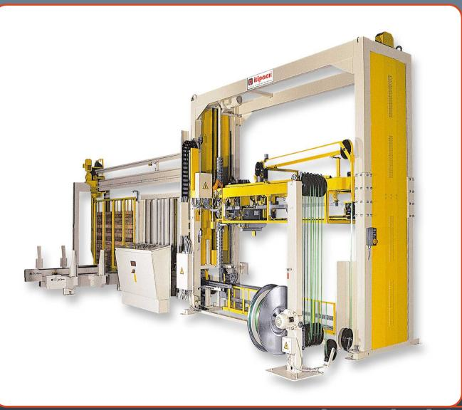
Strapping machine to strap chipboard panels. It is equipped with high tensioning system and with bottom wooden batterns applicators with powered magazine. Also it has top edge protector applicators. It is available with sealing head for polyester strap up to 19 mm. wide and 1.3 mm. thickness.
