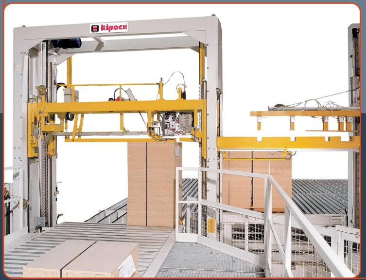
Strapping machine to strap chipboard panels. It is equipped with self-positioning system referred to pack height. It is available with sealing head for steel strap or for polyester strap.
