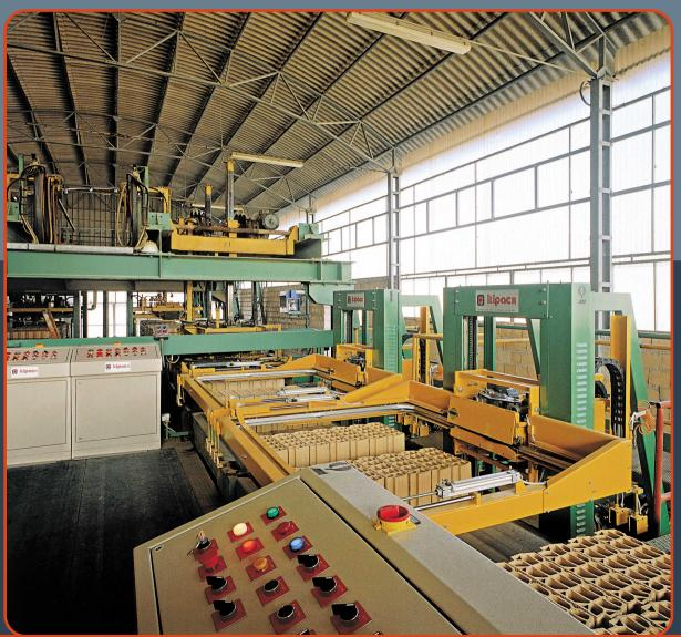
View of two fully automatic horizontal strapping machines for ceramic bricks, dual compaction closes pack whilst strap is applied.
