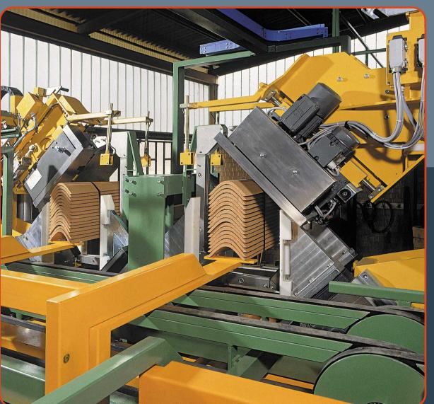
Automatic strapping machine, suitable for transversal strapping of roofing tile packs. It is equipped with pneumatic devices for compacting and alignment of packs during strapping cycle. The heads pivot to left or right according to pack inclination.
