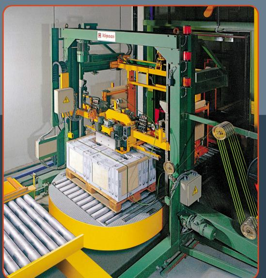
Fully automatic vertical strapping machine, travelling version, equipped with devices applying carton edge protectors having sizes 40x40x5 mm, L=700 mm and with turntable for crossed strapping. Suitable for palletised ceramic tiles.
