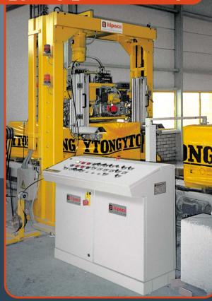
Vertical strapping machine with high tensioning capacity, it is equipped with automatic placing systems which dispense edge protectors size 60x60x4 mm. L = 120 mm. It is employed for strapping of prefab panels on building industry. This system is also available with side compression unit.
