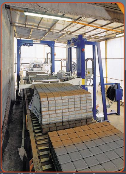
Strapping system formed of one horizontal strapping machine Mod. VKC/FG-N and one vertical strapping machine Mod. VKE/MRL, suitable for palletised concrete blocks.
