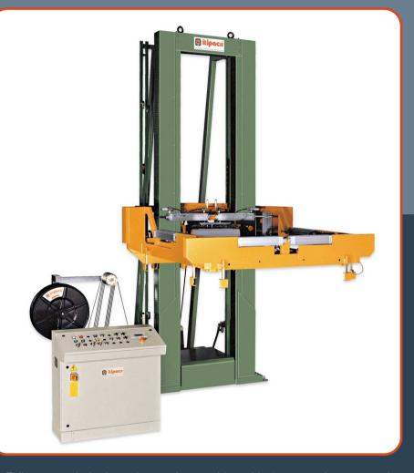
Fully automatic horizontal strapping machine with 4 pneumatic compression devices for palletised pack of tiles.
