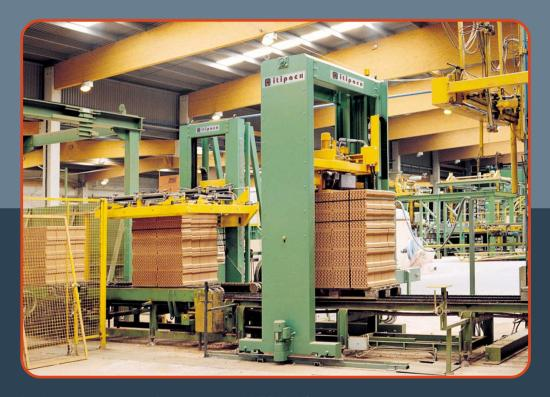
Double machine system for brick packs. VKE/MRLXO indexes along pack and applies vertical straps to each blade of bricks. The machine is fitted with a floating head for tension equalisation and can be adjusted for inclined straps. VKC/F4P compacts bricks blades together from all four sides and then applies the horizontal strap.
