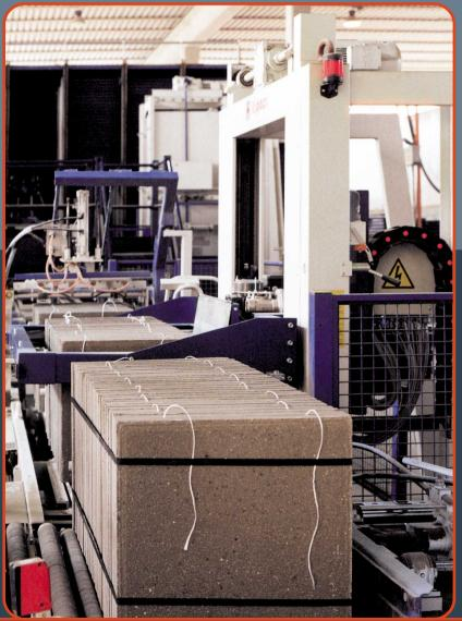
Horizontal strapping machine equipped with strap guide device for paving blocks.
