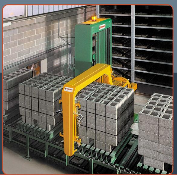
Robot machine for automatic vertical, horizontal and inclined strapping, It is suitable for concrete and paving block, and it is equipped with strap guide device. This machine enables horizontal and vertical straps to be applied using only one machine instead of the conventional two machine system.
