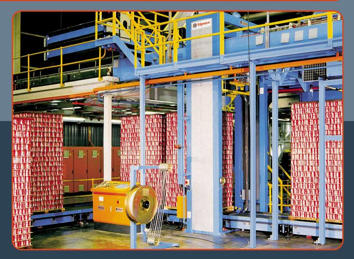
Automatic strapping machine to strap pallet of empty cans. It is equipped with 2 lances for introduction of strap through the pallet void and an adjustable compression bar up to 500 kgs.
