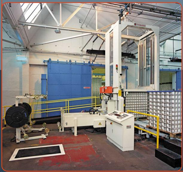
Strapping machine to strap pack of empty cans equipped with two sealing heads using polyester strap; stabilising and pressing bar of pack till 500 kgs. A smoke / fume extraction filter is also available.
