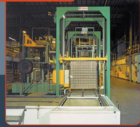
Automatic strapping machine to strap pallet of empty cans. It is equipped with movable lance for introduction through the pallet void and a side mounted head applying high tensile strap. With stabilising and pressing bar of pack till 500 kgs. A smoke / fume extraction filter is also available.
