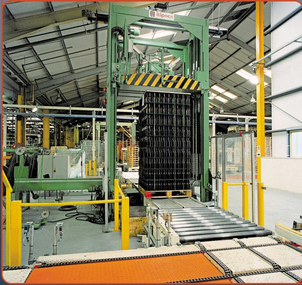
Compression strapping machine, maximum compression 5 T, for strapping glass bottles on pallet. It is equipped with 3 movable lances for introduction of strap through the pallet void and 3 sealing heads using polyester strap; It has a turntable to get cross strapping on pallet and an operative panel for a close dialogue between machine and operators, fully open to set up new strapping patterns. An 'in line' diagnostic unit is also available.
