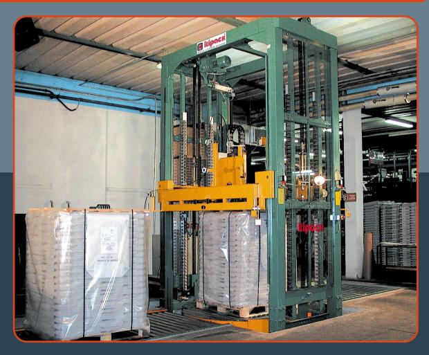
Compression strapping machine for vertical strapping of paper sacs on pallet, 2 Tons compression. It is equipped with two movable lances for introduction on the pallet and underfeed channels for strapping of packs without pallet. It has the self levelling compression platen system according to pack height and a turntable to turn the pack to apply cross strapping. The head moves on two vertical channels.
