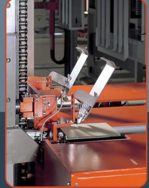
Compression strapping machine for corrugated carton equipped with 4 edge protection applicators, dimensions 200x200x5 mm, to protector the top of edges of the load being strapped. It owns 4 carton edge storages.
