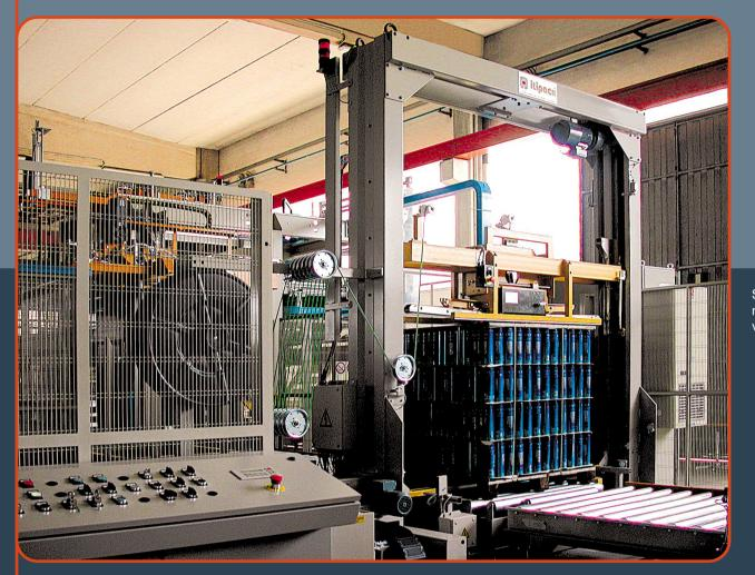
Strapping machine to strap cans on pallet. Equipped with movable lance for introduction of strap through the pallet void and top mounted head applying high tensile strap.
