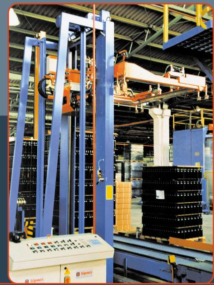
Horizontal strapping machine with 4 side compression devices for compression and strapping of glass bottles on pallet.
