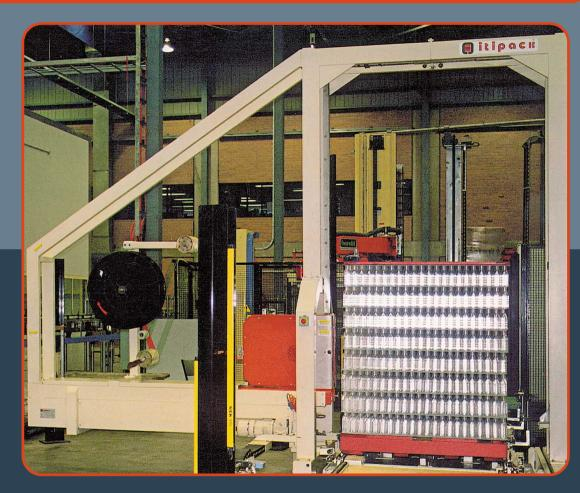
Strapping machine to strap PET bottles on pallet. Equipped with movable lance for introduction of strap through the pallet void and side mounted head applying high tensile strap. It gives equalised strap tension on the whole pack.
