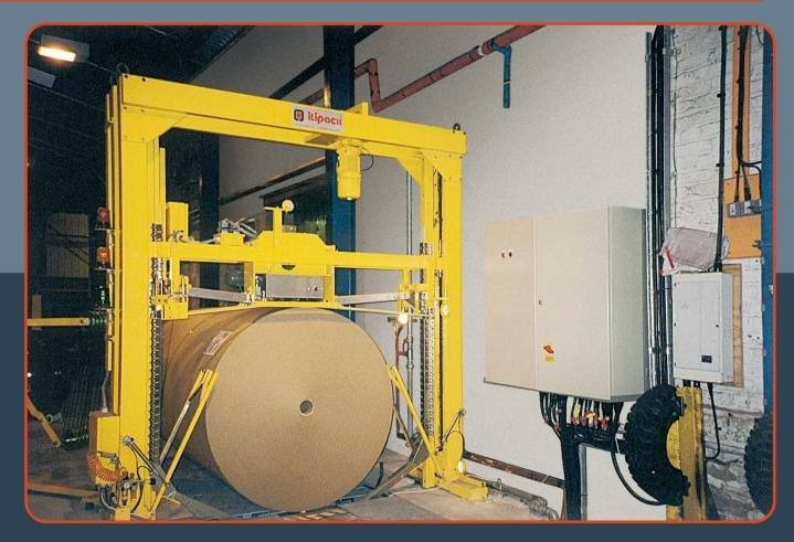
Circumferencial strapping machine for paper rolls, provided with strap guide arms for the precise positioning of the strap on the roll. It is equipped with sealing head for use with polyester strap.
