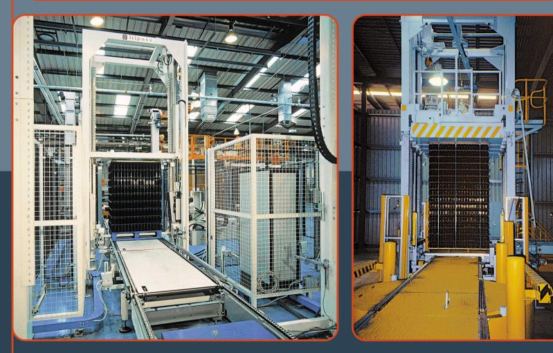
Compression strapping machine, maximum compression 5 T, for strapping glass bottles on pallet. It is equipped with 3 movable lances for introduction of strap through the pallet void; 2 sealing heads working on 3 channels using polyester strap. It has an operative panel for a close dialogue between machine and operators, fully open to set up new strapping patterns. An 'in line' diagnostic unit is also available.
