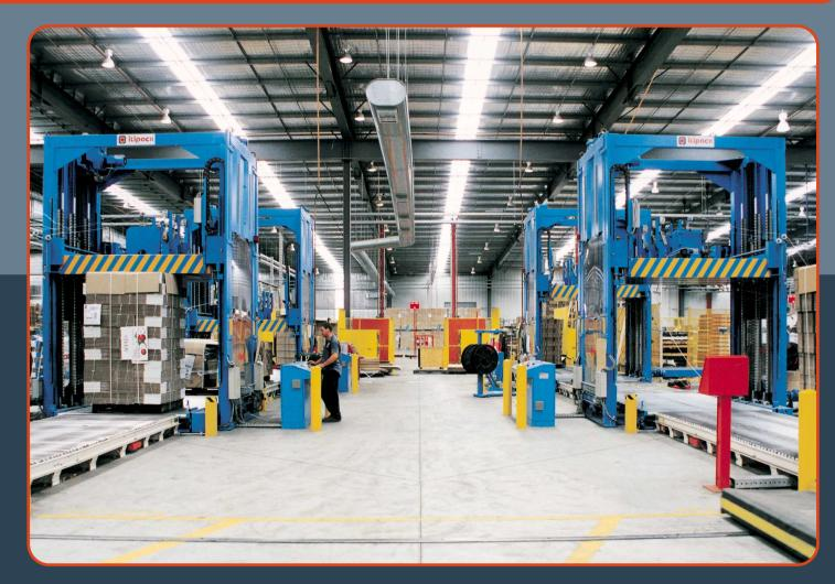
Packaging line on corrugated board packages. It is realised by four compression strapping machines – compression till 5 Tons. It gives high production capacity and maximum strapping flexibility reached by an advanced technology and a close rapport between machine and operator.
